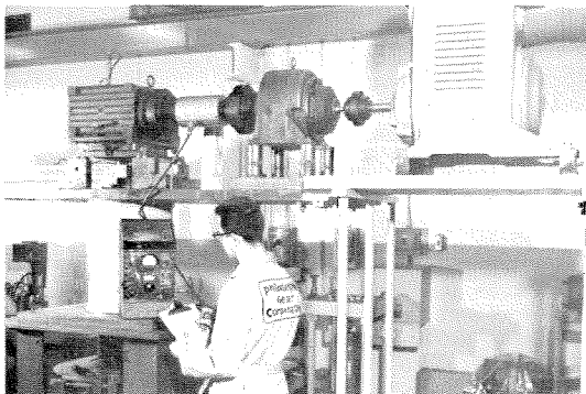
Worm gear reducer on efficiency test in laboratory.
