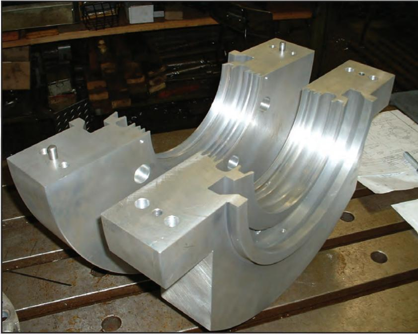
Other causes of gearbox failures can be attributed to oil leaks. To prevent this in one application, this “super” seal was developed by Philadelphia Gear engineers to solve leakage problems.
