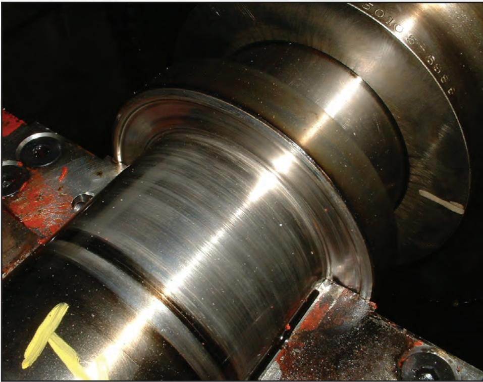
Proper maintenance and periodic inspection are important to preventing a power plant's mission critical components such as gearboxes from failing. Shown is a damaged No. 1 shaft thrust collar on an accessory gearbox. To prevent this type of failure, axial movement checks are part of the plant's preventive maintenance.
